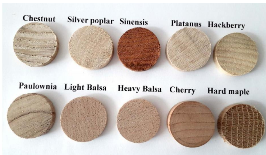
Fig. 3. Photograph of different hardwood specimens. Source: (Kolya and Kang, 2020)
